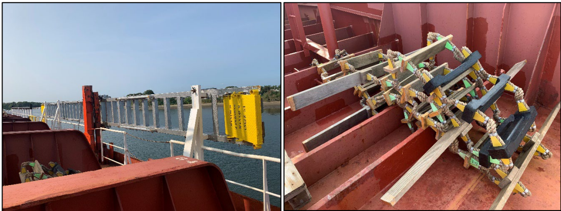
Figure 3. Photos of accommodation ladder (left) and pilot ladder (right) in stowed position, onboard the MTM DUBLIN taken September 27, 2023 (Source: USCG).
